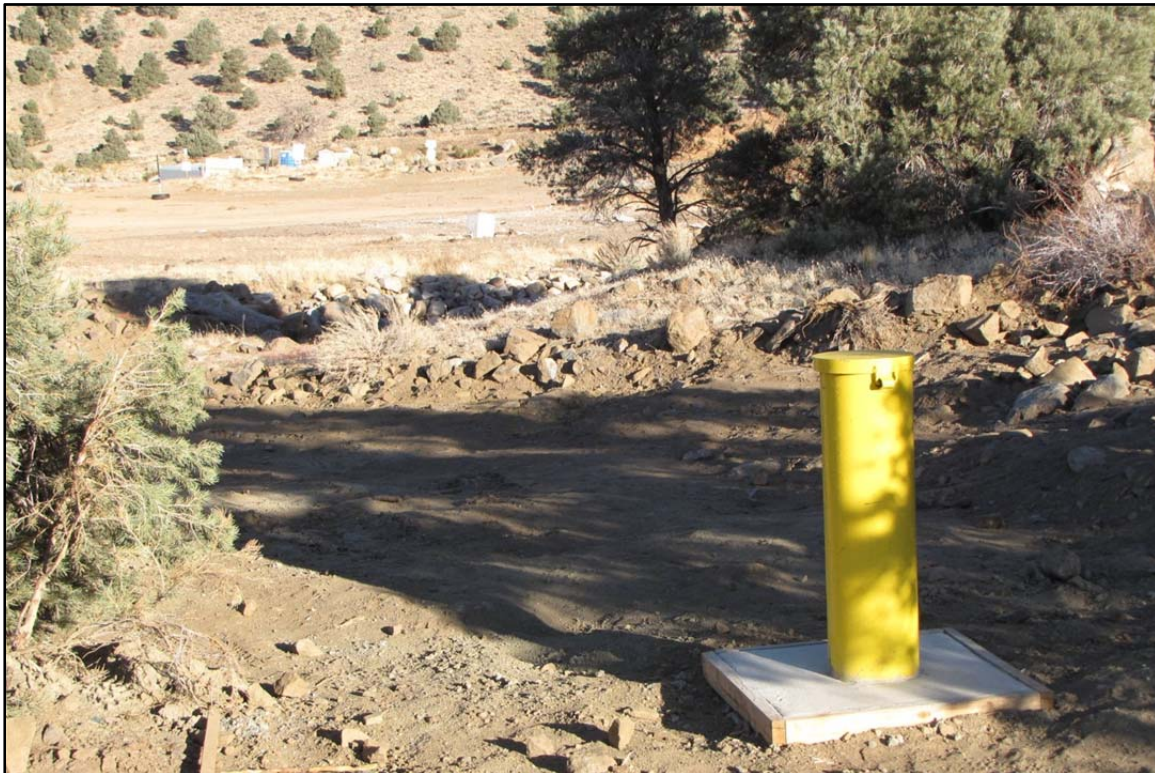
Plate 2-10. LFG monitoring well GW-4 with landfill and transfer station in background (view north).
