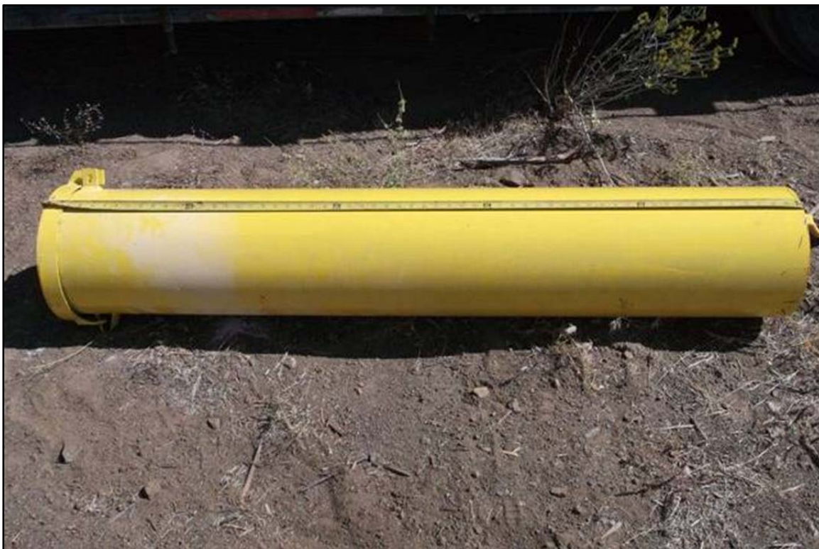
Plate 1-4. Typical five-foot long painted steel surface completion monument with locking cap.
