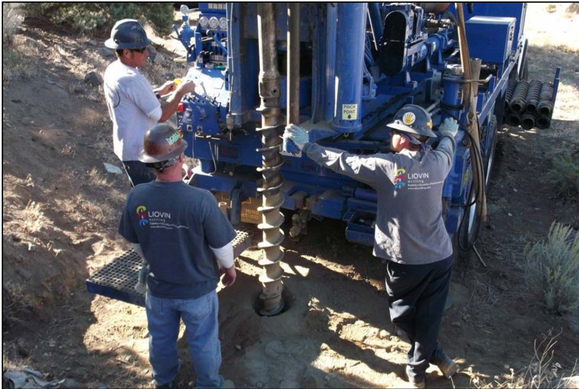
Plate 1-3. Truck-mounted hollow-stem auger rig over borehole (WK LF GW-1, view south).
