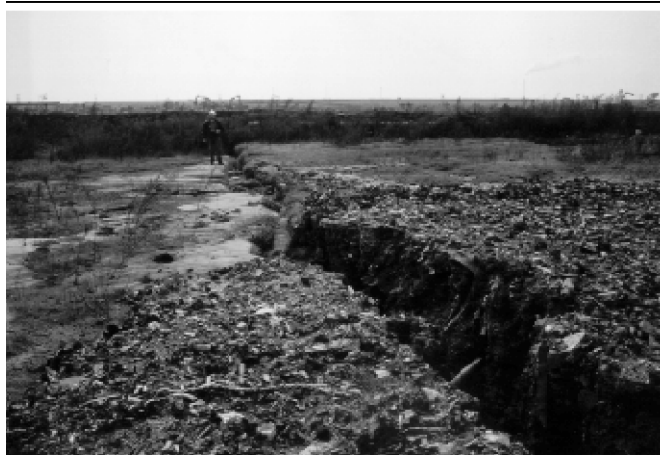
Figure 1. Sand liquefaction boil with some garbage ejecta (photograph courtesy of Dr. L. Harder).
