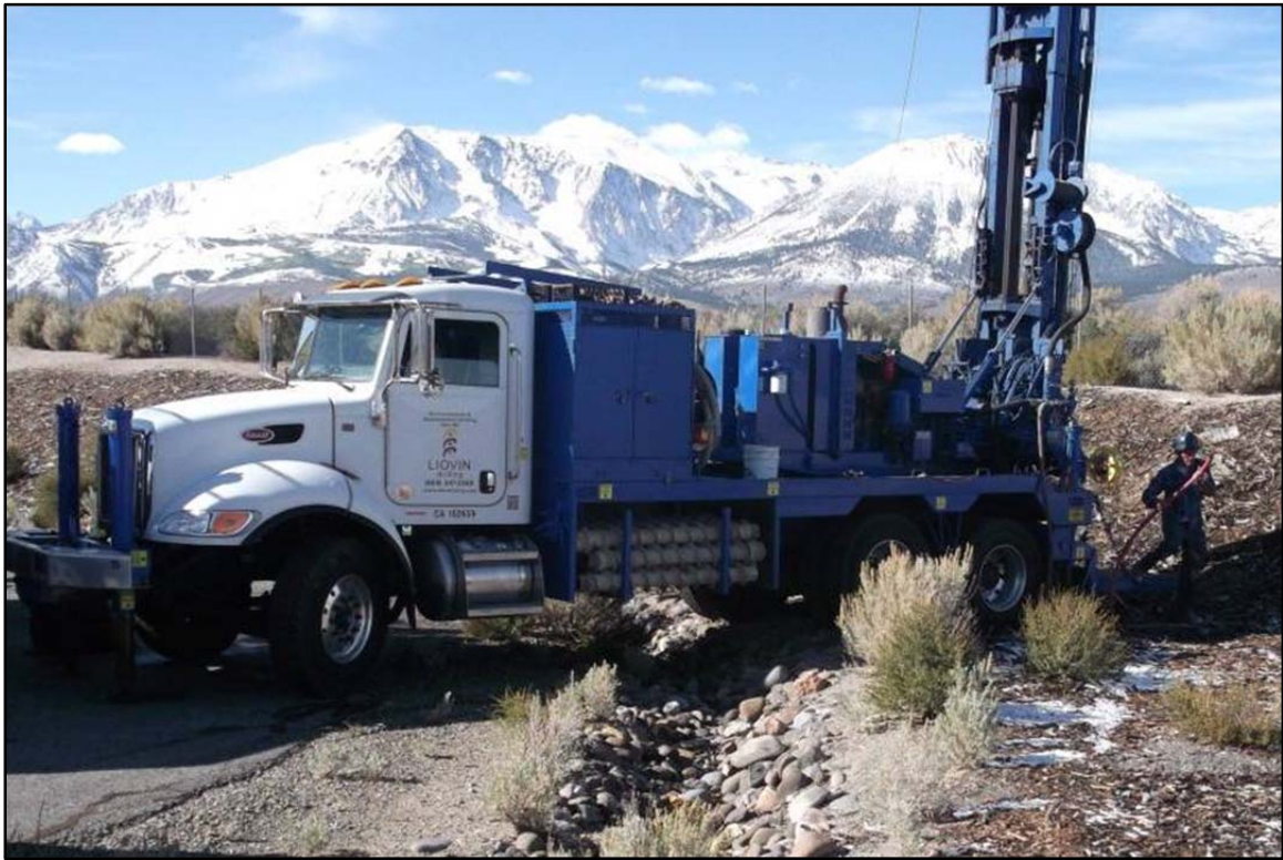
Plate C-1. Truck-mounted hollow-stem auger rig over borehole (GW-1, view west).
