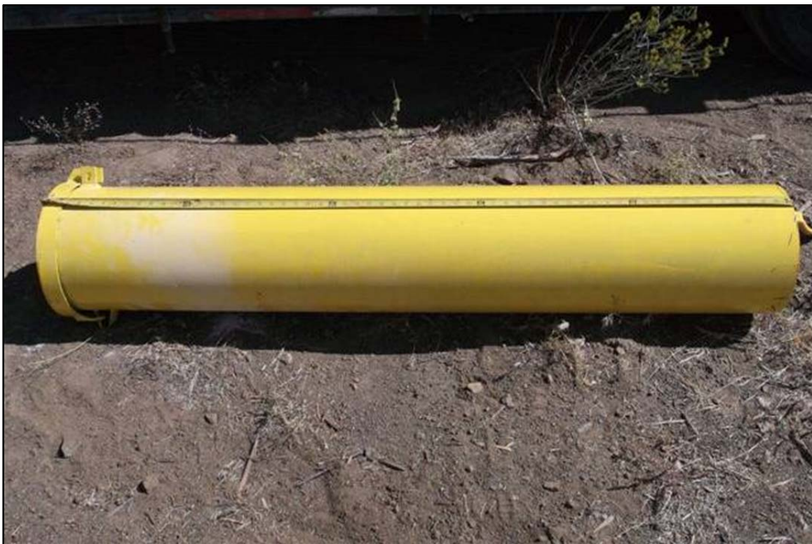
Plate C-4. Typical five-foot long painted steel surface completion monument with locking cap.
