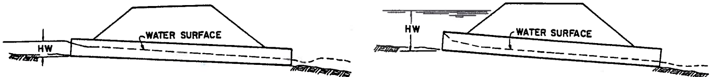
TYPICAL INLET CONTROL CONDITIONS
