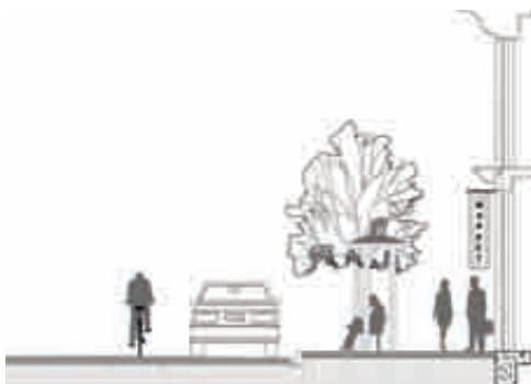
Fifteen foot sidewalks create area for high levels of pedestrian activity.
