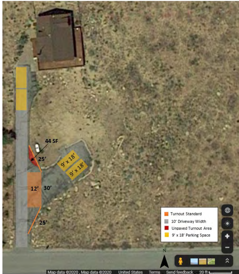
FIGURE 6: DRIVEWAY TURNOUT ANALYSIS
