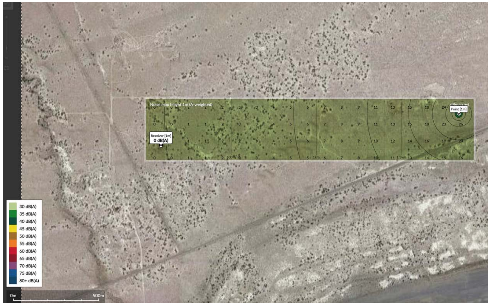
FIGURE 3- NOISE CONTOUR DEPICTING dBA LEVEL AT THE PROJECT'S WESTERN PARCEL BOUNDARY (SIDE WITH THE CLOSEST SENSITIVE RECEPTOR)
