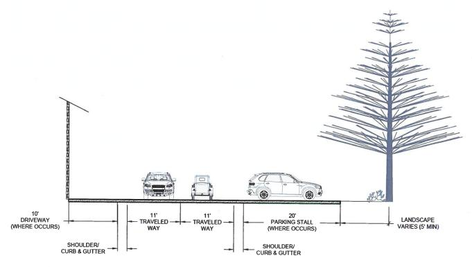
Figure 12: Typical Internal Circulation Road Section 1
